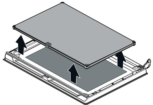
6. Remove the holders to separate the two middle panels from one another.
