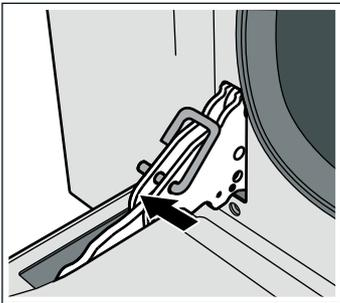
3. Using both hands, lift the bottom of the inner panel slightly until the fastening pins come out of the holder.
