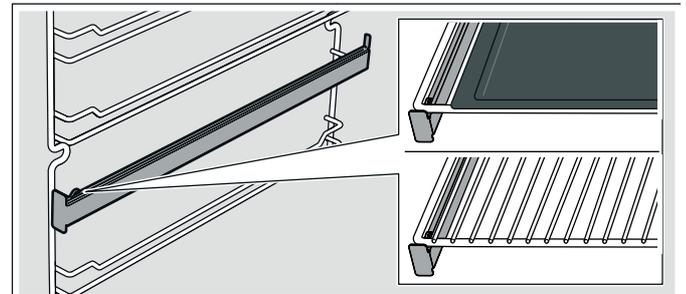
**Note:** The rotary spit must be inserted on level 1. In this case, move the pull-out rails for the baking tray and the baking and roasting shelf to the four upper levels.
