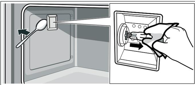
7. Replace the oven light bulb with a bulb of the same type:
