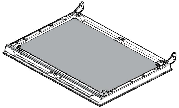
**Note:** The two middle panels are not fastened using retaining pins; instead, they are held in place using holders.
