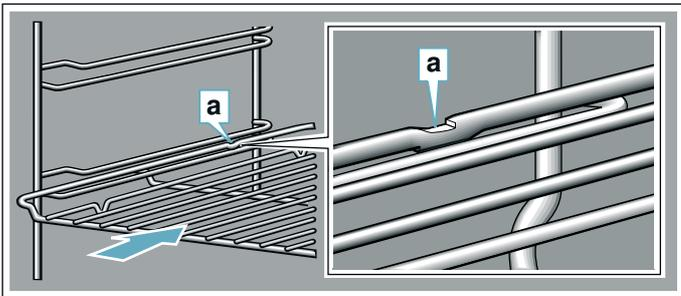
When inserting baking trays, ensure that lug **a** is at the rear and is facing downwards. The sloping edge of the accessory **b** must be facing towards the appliance door.
