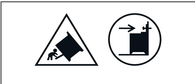
**Warning:** In order to prevent tipping of the appliance, this stabilizing means must be installed. Refer to the instructions for installation.
